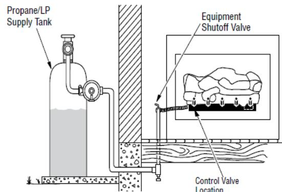
**Figure C - External Regulator with Vent Pointing Down**
