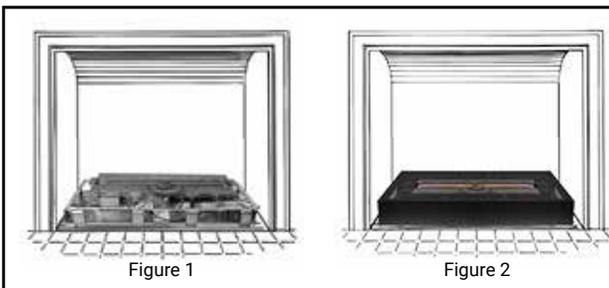
Place Bedrock burner in your fireplace centering the base front to back and side to side. Centering the base allows the case to easily slide over the top of the base. (Figure 1)
