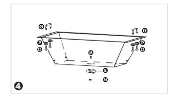
Use 1 Screw with Washer to attach the Lid Handle to the top of the Fire Bowl Lid .
