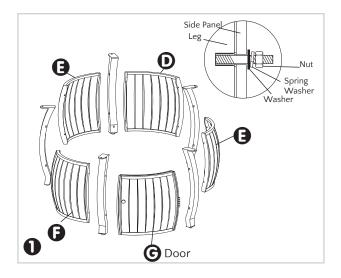
Once all **Panels** and **Legs** are bolted together, carefully turn the assembled table base upside-down.
