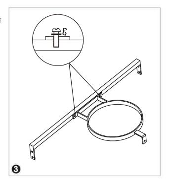
Attach Tank Support Bar ① to Door Frame Leg ③ and Support Leg 1 ⑤ by aligning holes at each end of Tank Support Bar with holes at the bottom of Door Frame Leg and Support Leg 1. Place a Washer ② on each of 4 Bolts ② and insert into holes. Tighten with Hex Key ③.
