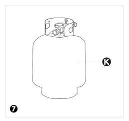
A dented, rusted or damaged propane cylinder may be hazardous and should be checked by your cylinder supplier. Never use a propane cylinder with a damaged valve connection.
