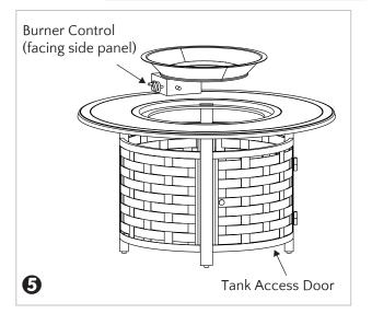
Pour the Fire Glass ① around the Burner. Be careful not to obstruct the pilot light housing. Put the Removable Burner Cover ② on the Burner when not in use. When the fire pit is not in use or after use, when the fire pit has cooled COMPLETELY, cover it with the Protective Cover ③. DO NOT PUT THE PROTECTIVE FIRE PIT COVER ON A HOT FIRE PIT.
