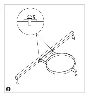
Attach Tank Support Bar ① to Door Frame Leg ② and Support Leg 1 ③ by aligning holes at each end of Tank Support Bar with holes at the bottom of Door Frame Leg and Support Leg 1. Place a Washer ② on each of four Bolts ② and insert into holes. Tighten with Hex Key ③.
