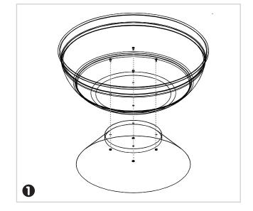
Attach Handle (A) to Fire Screen (B) with a Nut (1). Securely tighten.
