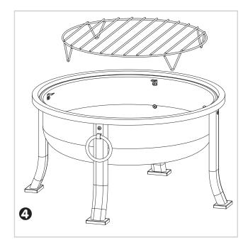
Place the Fire Screen ③ on top of the fire pit. Make sure to use the Fire Tool ⑥ to add or move logs or for removing/replacing the Fire Screen.
