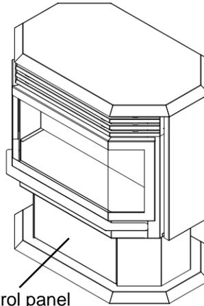
Push here to open the manual control panel
