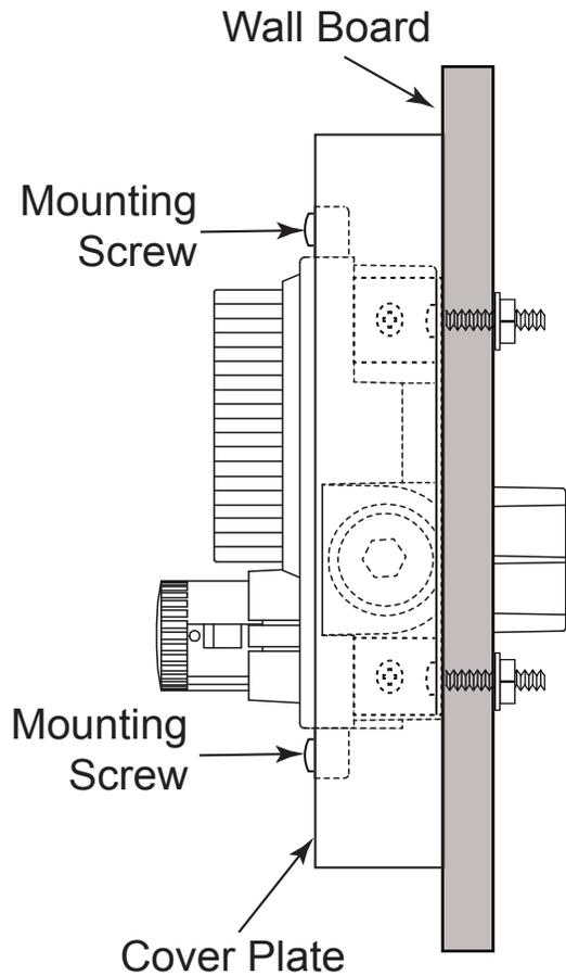
**Fig. 6** Side view of ESTOP mounted into wall.
