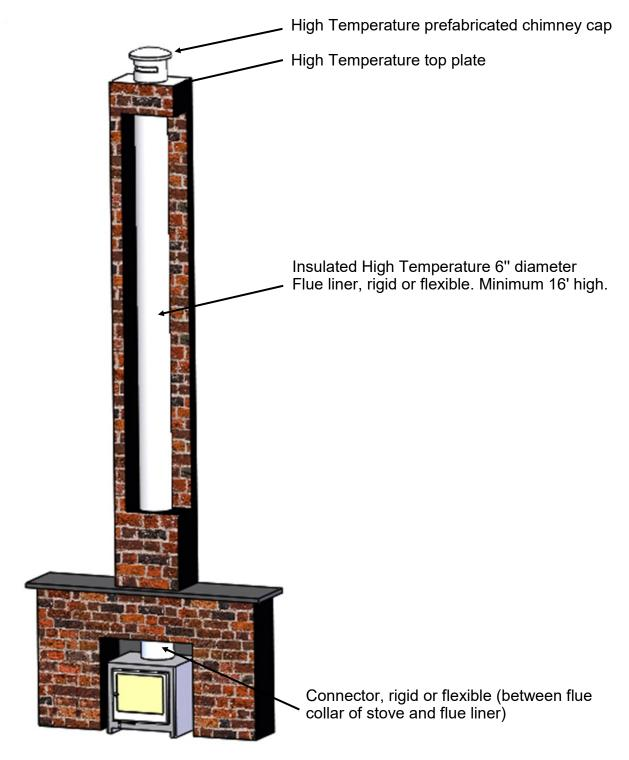
Sample installation into existing chimney.
