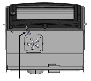
Minimum Closed Position (Lever In LH Position)
