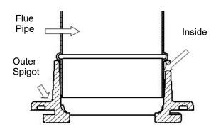
Fig. 1. Flue & Spigot Fitting
