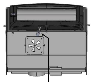
**Fully Open Position (Lever In RH Position)**
