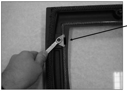
Fig. 8. Tightening The Glass Clip
