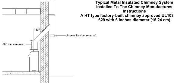
Instructions A HT type factory-built chimney approved UL103 or ULC 629 with 6 inches diameter (15.24 cm)
