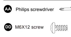
8. Line up the screw holes on the table (C) with the left and right side panels. Use 4 M6X12 screws to attach the table tightly.
