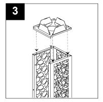
6. Install the Glass Tube inside the Decorative Plates, holding it at an angle. First set the top of the tube in the opening of the Fixing Plate(3)
