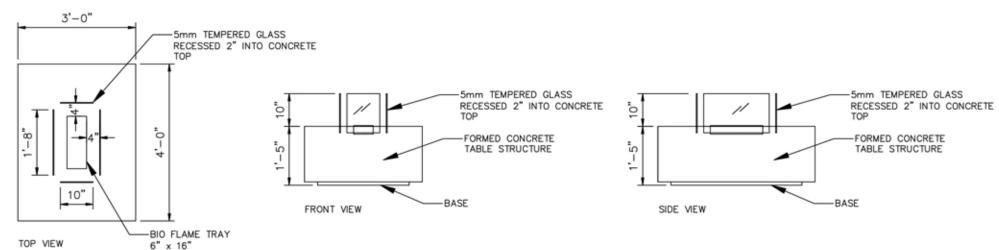
\*Dimensions may vary by 2% (plus or minus) due to material attributes. Template not provided. The Bio Flame recommends using the actual fireplace or burner model when making final cut out.
