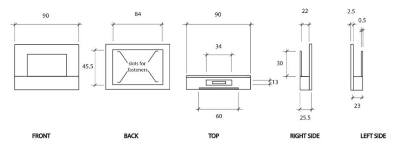
\*Dimensions may vary by 2% (plus or minus) due to material attributes. Template not provided. The Bio Flame recommends using the actual fireplace or burner model when making final cut out.
