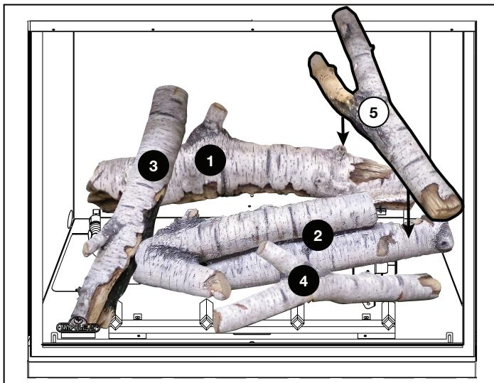
5. Place the bottom right side of Log #4 on Grate Post #4 under Log #2. Ensure the log engages with the locating bracket. Rest the "Y" end between Grate Post #2 & #3 and engage with main bar.
