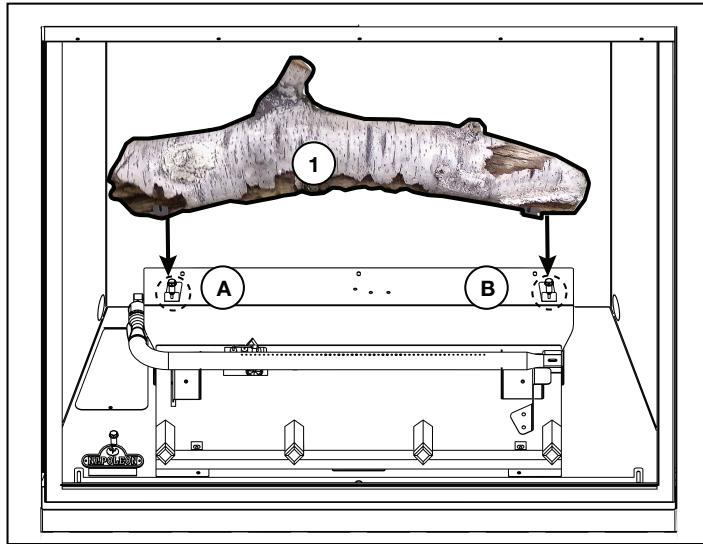
1. Install the Locating Bracket onto the media tray. The bracket can be found in the manual bag.
