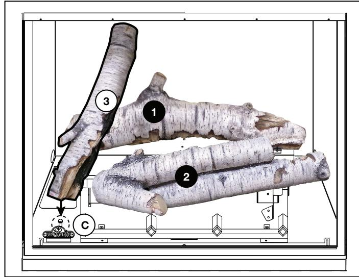
3. Place the scar on the "Y" of Log #2 on Grate Post #2, resting the opposite end on the locating bracket. Ensure the log does not cover any burner ports.
