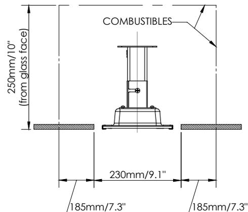
1. Prepare ceiling cut-out with dimensions from images on P.9 to fit ceiling recess frame (a). Heater must be installed with heater surface at least 2400mm above the floor level, with 500mm clearance to the nearest wall on all sides of the heater. Minimum distances to combustibles within cavity must be according to **only one** of the two options shown.
