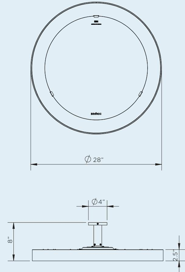
Measurements displayed within this document are minimum requirements for installation. Bromic takes no responsibility for incorrect or non-compliant installations. All measurement in this document are displayed in inches.
