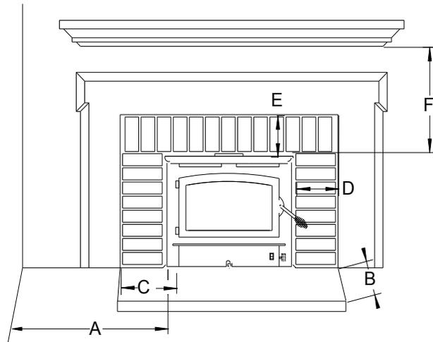
1. The hearth must be of masonry construction and must extend a minimum of 16" in front of firebox opening and a minimum of 8" to either side of firebox opening.
