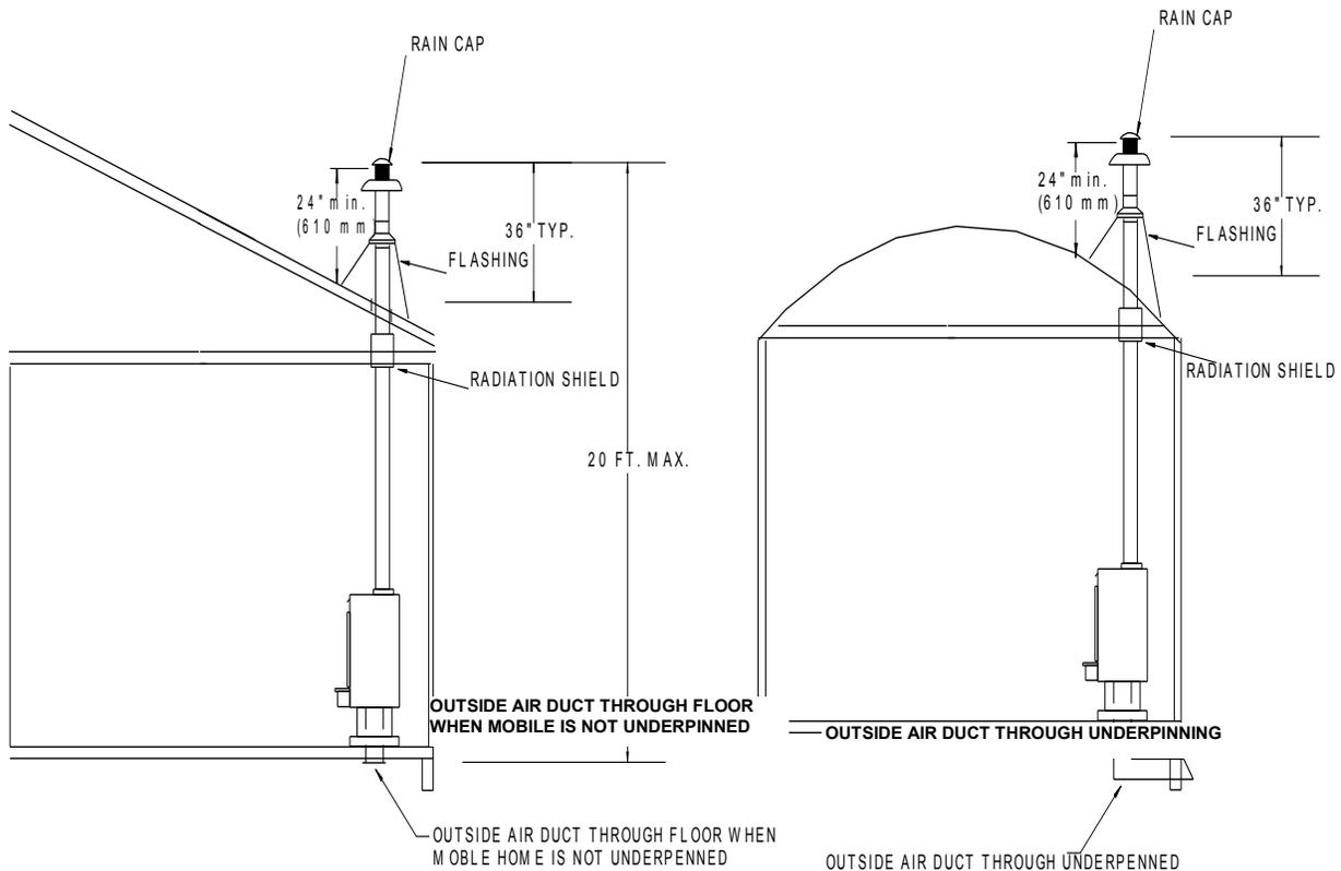
**Ceiling Exit (Using Close Clearance Listed Chimney)**
