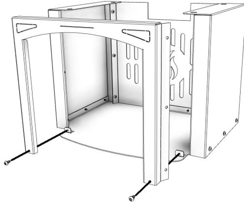
5. Secure the front panel of the pedestal to the left and right side panels of the pedestal using a total of six (6) # 10 screws as shown. NOTE: The back pedestal panel was removed in this image for clarity purposes only. Do Not remove the back pedestal panel when installing the front pedestal panel.
