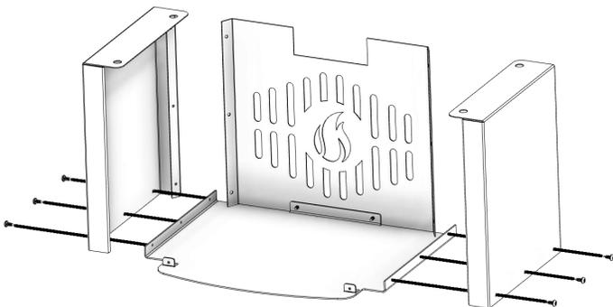
3. Secure the left and right side panels of the pedestal to the pedestal back using a total of six (6) # 10 screws as shown.
