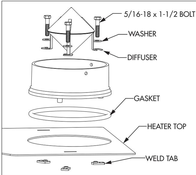
Above is an illustration of the installation of the flue collar and diffuser. The installation of this diffuser is critical for the proper functionality of this appliance. Failure to install this diffuser can result in a possible over fire situation. This diffuser is critical to the proper functionality for the cleanest burning fires in your stove. **FAILURE TO INSTALL THE DIFFUSER CAN RESULT IN FIRE, PROPERTY DAMAGE AND/OR DEATH.**
