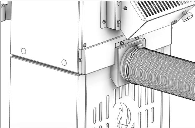
Slide the hose clamp over the aluminium flex pipe. Then slide the flex pipe over the air intake tube of the stove. Next tighten the hose clamp over the end of the aluminium flex hose.
