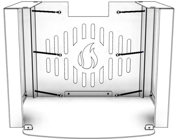
4. Attach the front panel of the pedestal to the pedestal base using two (2) # 10 screws.
