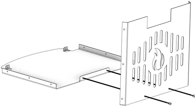
2. Attach the left and right side panels of the pedestal to the pedestal base using a total of six (6) # 10 screws.
