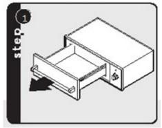
Pull out drawer assembly until fully extended
