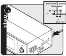
Feed supply cord up through hole in rear of warming drawer.
