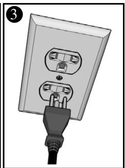
Plug into a grounded three-pronged outlet. The DRAW COLLAR runs at 120V, 500 Watts.
