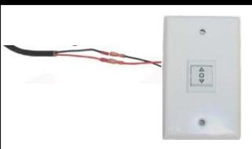
CONNECT THE TERMINALS FROM THE CLC-BLOCK TO THE TERMINALS OF THE BATTERY PACK AND INSTALL THE BATTERIES. THE ROCKER SWITCH WILL THEN TURN GAS FLOW ON/OFF.
