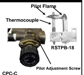
IMPORTANT: These controls are factory preset and will not normally require additional adjustment of the pilot flame. If field adjustment of the pilot flame is required, adjust using the pilot adjustment screw. The 90 degree pilot should produce 2 flames about 1-1 ½" in 2 directions. One flame should come towards the front of the firebox to ignite the burner and the other, wrapping around the thermocouple to ensure proper valve operation.
