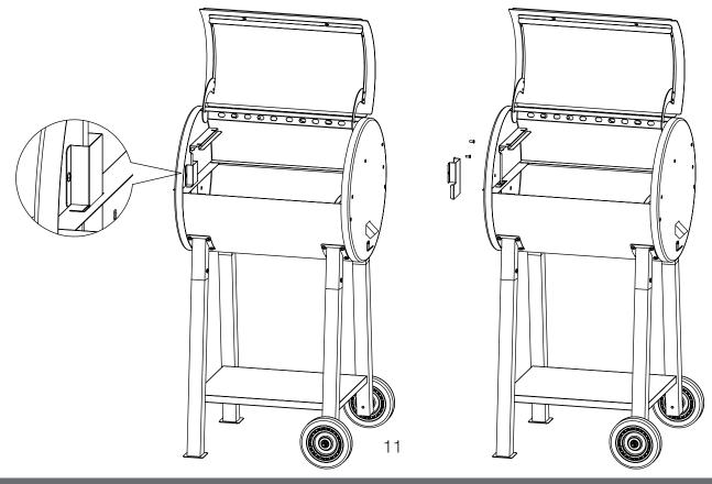
• Assemble the top section of the hopper as shown. Note the positions of Panels (2), (3), (4), and (5). Secure the panels to each other using 8 Screws (F).
