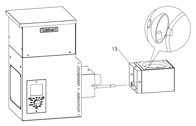
• With the hot rod in place, re-install the screw removed in Step 11 to secure the hot rod.
