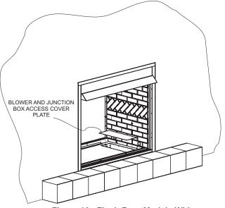
Figure 16 - Flush Face Models With Raised Hearth Extensions
