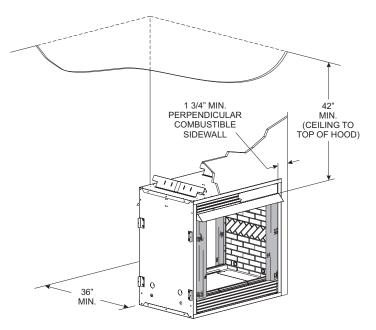
Figure 1a - See Through Firebox Clearances
