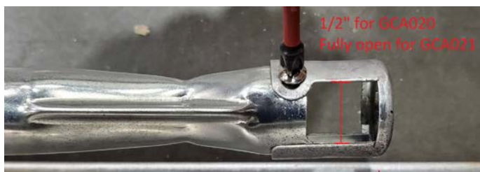
Figure 13.c primary air adjuster
