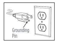
A 15 Amp, 120 Volt circuit is required. A dedicated circuit is preferred, but not essential in all cases. A dedicated circuit will be required if, after installation, the circuit breaker trips or the fuse blows on a regular basis when the heater is operating. Additional appliances on the same circuit may exceed the current rating of the circuit breaker.
