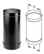
Use for a single-wall connector pipe. Requires 18" clearance to combustibles. Subtract 1 ¼" from length to calculate the installed length.
