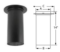
Used to adapt DuraBlack pipe to 6" - 8" Ceiling Support Box, including DuraTech, DuraPlus, and DuraTech Premium systems. The Slip connector can also be added to 6" - 8" DuraTech finishing collar. Adds 3"-13" of length to rigid pipe. Provides a strong mechanical connection.
