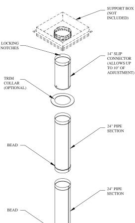
**Step 2.** If you are installing the optional Trim Collar, slide the Trim Collar upwards over the Slip Connector, until it is next to the bead. Using the two pre-punched holes in the Trim Collar as a guide, drill two 1/8" diameter holes in the Support Box. Screw the Trim Collar to the support box, using the two sheet metal screws provided with the kit.
