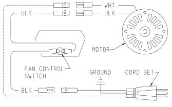
IF ANY OF THE ORIGINAL WIRE AS SUPPLIED WITH THIS UNIT MUST BE REPLACED, IT MUST BE REPLACED WITH 125°C 2/64 INSULATION WIRE OR ITS EQUIVALENT.
