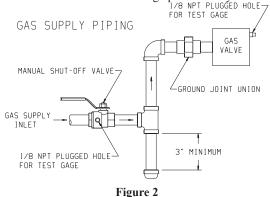
Method of Installing a Tee Fitting Sediment Trap
