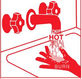
Water temperature over 125°F can cause severe burns instantly or death from scalds. Children, disabled and elderly are at highest risk of being scalded. See instruction manual before setting temperature at water heater. Feel water before bathing or showering. Temperature limiting valves are available, see manual.
