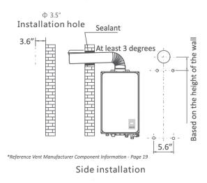
Indoor unit must be installed with CAT 3 vent pipe in acc ordance with v ent supplier/ Manufacturer in acc ordance with loc al code. Owner must refer to vent manufacturer's instructions and specifications. Z-Flex information can be found at www.novaflex. com, please refer to page 32 for additional links.
