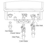
NOTICE: The hot and cold pipes should be insulated as shown help to provide additional freeze protection
