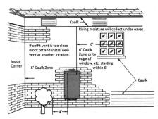
WARNING : Moisture in the flue gas will condense as it leaves the vent terminal. In cold weather this condensate can freeze on the exterior wall, under the eaves and on surrounding objects. Some discoloration to the exterior of the building is to be expected. However, improper location or installation can result in severe damage to the structure or exterior finish of the building. Code requirements are subject to change and may vary by location.
