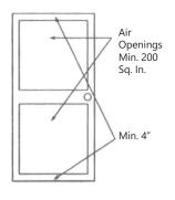
A confined space is one having a volume of less than 50 cubic feet per 1,000 BTUH of the aggregate input of all appliances within that space.
