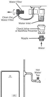
If a water heater is installed in a closed water supply system, such as one having a backflow preventer in the cold water supply line, means shall be provided to control thermal expansion. Contact the water supplier or local plumbing inspector on how to control this situation. Install a shutoff valve near the inlet of the water heater for service and draining purposes.
