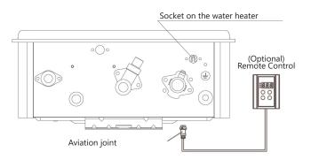
2. For two controls: First, cut off the aviation joints on the two controllers, plug one into the socket on the water heater (length is dependent on your requirements), and throw away the other. Then connect the wires of the aviation joint to the inlet wire of the connector, and connect the two remote control to the outlet wires of connector.
