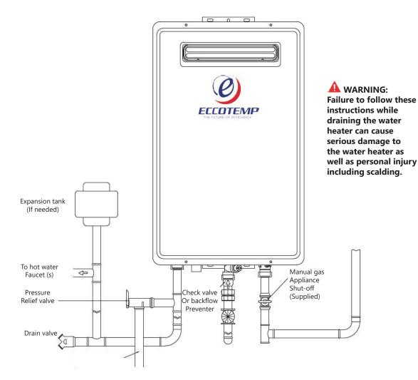
Below are instructions for draining water out of the water heater.
