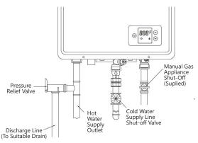
**NOTICE:** Local codes govern the installation of relief valves. If local codes require that a temperature and pressure relief valve should be installed the manufacturer recommends a type 40XL Watts T&P relief valve or an equivalent model be used.
