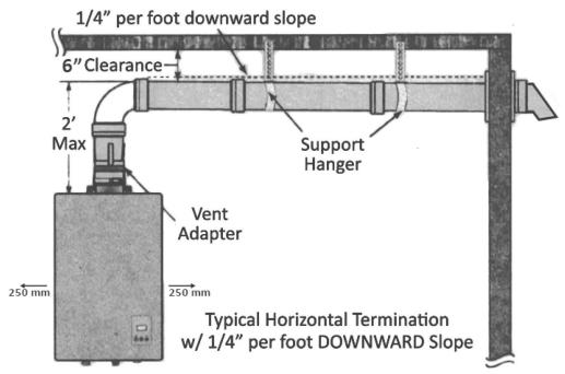
WARNING: Use UL approved Category III vent material only. No other vent material is permitted. Owner must refer to vent manufacturer's instructions and specifications. Z-Flex information can be found at www.novaflex.com, refer to page 32 for additional links.
