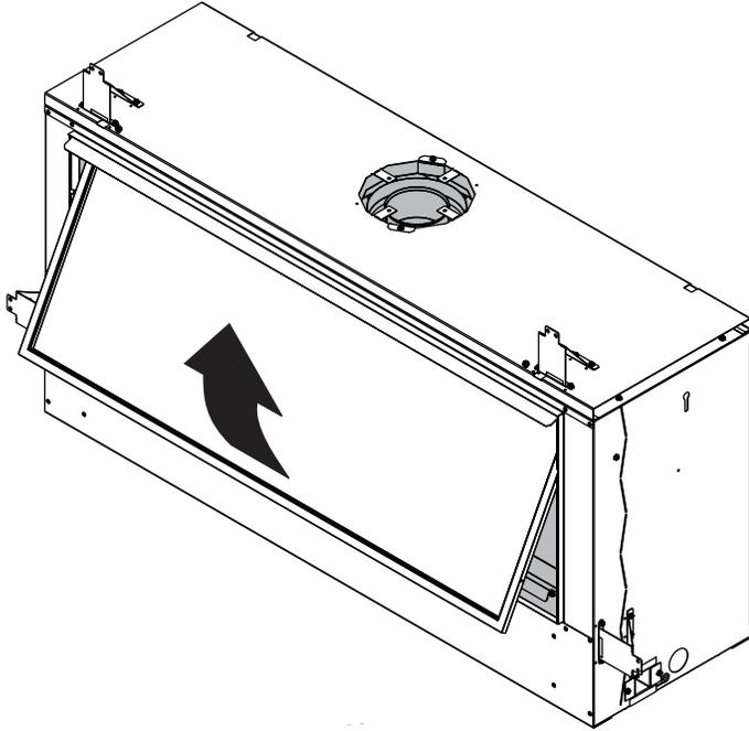
Tilt up on screen until top edge hits against Glass Frame. Continue to pull up until screen pops loose from firebox opening flanges.
