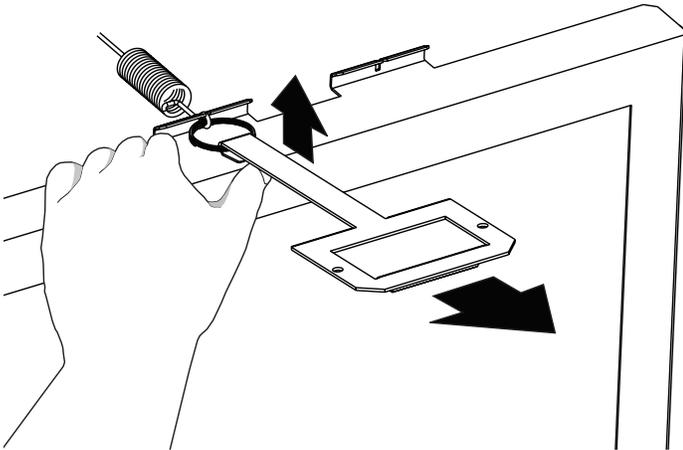
Pull Spring-Latch Ring away from the Glass Frame with right hand using Spring-Latch Tool (approx. 1/2" - 3/4"), and push up with left thumb to release the Spring-Latch from the Glass Frame Clip.
