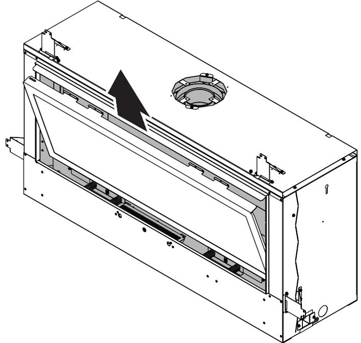
Tilt Glass Frame away from unit, enough to clear top lip, and pull forwards to remove.
