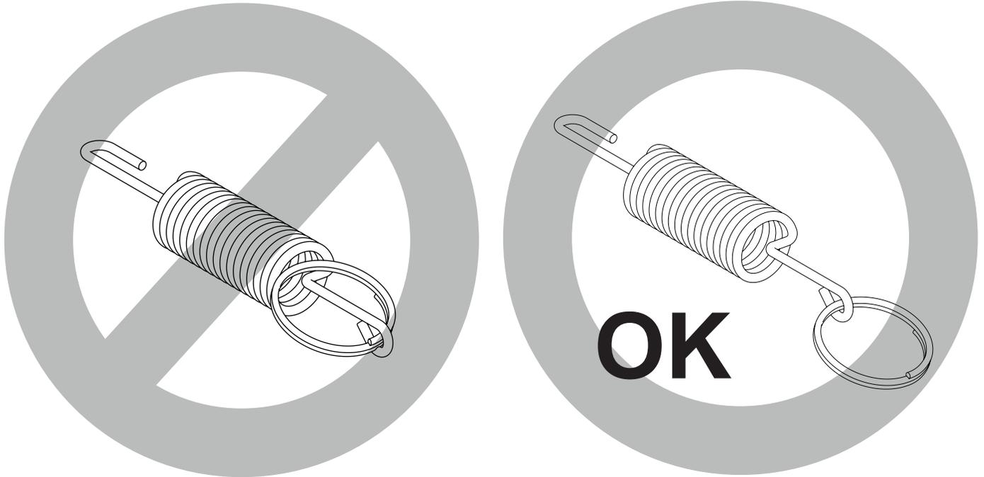
When installing the Glass Frame, do not pull on the Spring-Latch Ring if the ring is flipped backwards as shown above. Flip the ring forwards with your fingers or the Spring-Latch Tool before pulling on the Spring-Latch.
