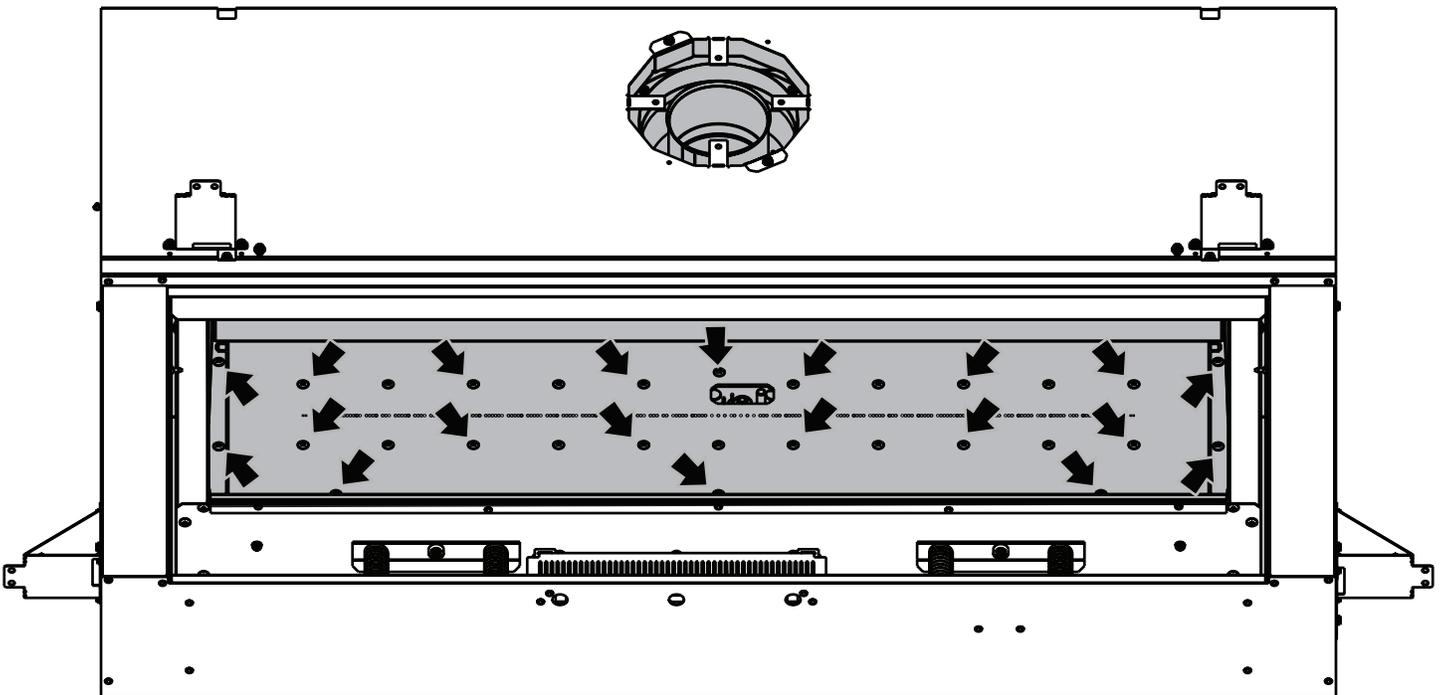
To access the burner, only the screws pointed out above need to be removed. The other burner surround screws may be left in place.
