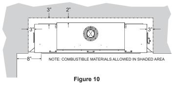
The minimum clearance from bottom of the fireplace to ceiling is 65 inch.
