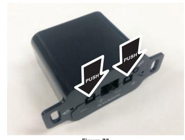
5. With the batteries already installed in the Transmitter, push the On button. The Receiver will beep four times to indicate the Transmitter's command is accepted and sets to the particular code of that Transmitter. The system is now initialized.
