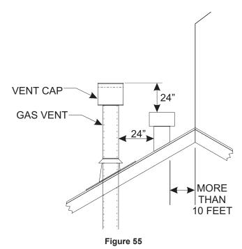
Note that for steep roof pitches, the vent height must be increased. In high wind conditions, nearby trees, adjoining roof lines, steep pitched roofs, and other similar factors can result in poor draft, or down-drafting. In these cases, increasing the vent
