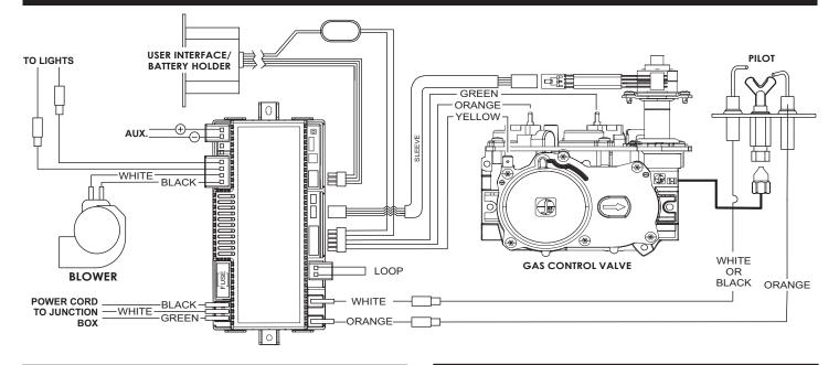
If any of the original wire as supplied with this fireplace must be replaced, it must be replaced with equivalent gauge and temperature rated wire.
