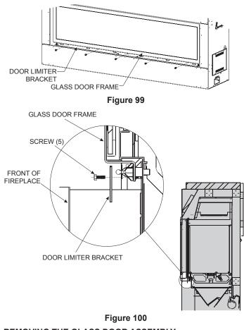
**REMOVING THE GLASS DOOR ASSEMBLY** Locate the glass door tool (secured to the top of the fireplace for shipping). Use the tool as a lever to release the bottom of the glass door as shown in **Figure 101**. **NOTICE:** The glass door is secured to the top of the firebox with tabs that allow it to pivot outward at the bottom. The bottom of the door frame engages into the four bullet type retainers.
