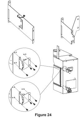
Secure fireplace to framing with nailing flanges. Preset depth to suit facing material (flush or 1/2 inch set back depths).
