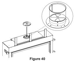
**NOTICE:** When installing flue restrictor, install with screw pointing downward.
