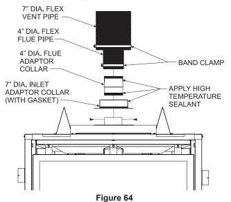
Once the lower connections are made and the flex pipe is secured with support bands as required (3 feet minimum between supports) then the roof flashing can be installed. See Figure 65.
