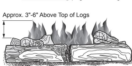
**Figure 25 - Correct Burner Flame Pattern**
