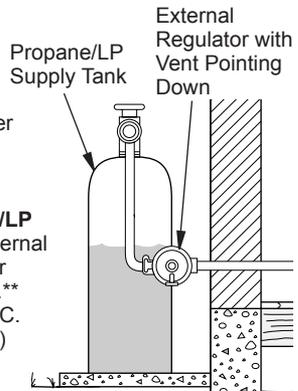
**Figure 14 - External Regulator with Vent Pointing Down**
