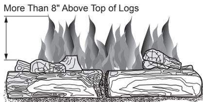
**Figure 26 - Incorrect Burner Flame Pattern**
