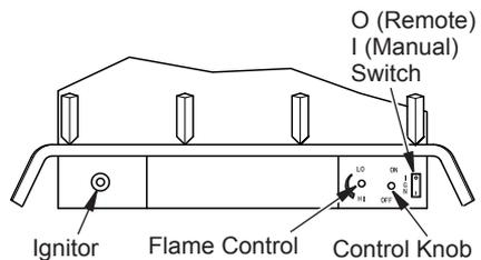
**Figure 19 - Ignitor Button and Control Knob Locations**
