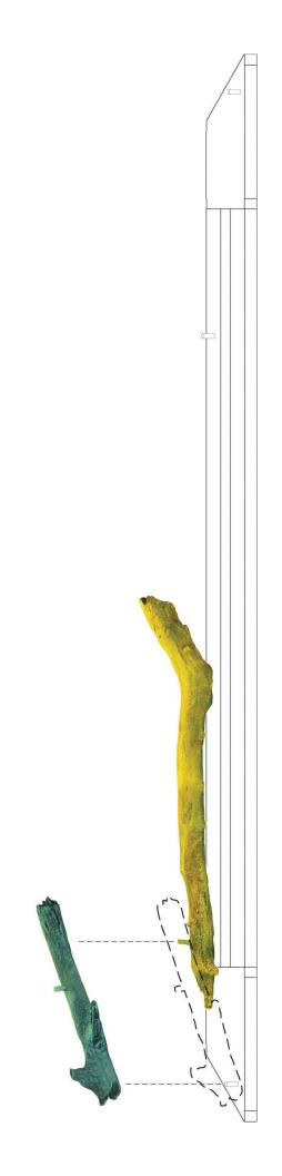
3. Place Log C onto pin on Log B and angle to the front of the burner so it rests on the front glass support screen.
