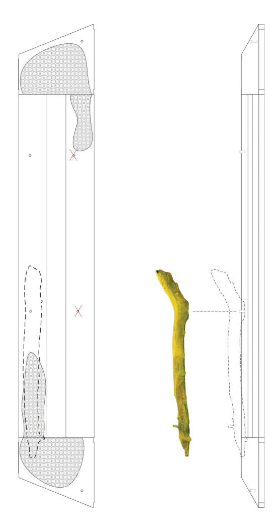
2. Place Log B onto Front Left Pin and the pin on Log A.
