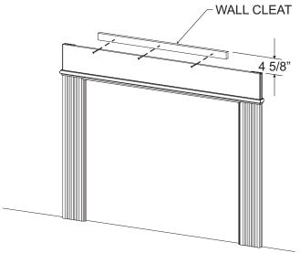
8. Align and attach Mantelshelf to 1" X 2" X 42" wall cleat with finishing nails.
