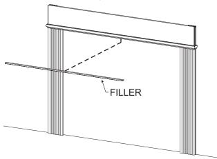
Attach vertical cove to inside edge of fluting with finishing nails. The back surface of vertical cove must be flush with front surface of decorative stone or marble. The vertical cove will hold the decorative stone or marble in place.
