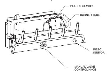
Manual Valve for VFDM Series Figure 18
