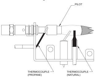
Incorrect Flame Pattern for VFDT & VFDM Figure 23
