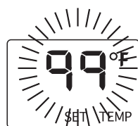
SCREEN AT HIGHEST THERMO SETTING
