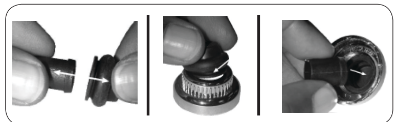
Fig. 24-5 Rubber cap replacement
