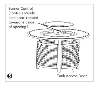
Pour the Fire Glass around the Burner. Be careful not to obstruct the pilot light housing. Put the Removable Burner Cover on the Burner when not in use. When the fire pit is not in use or after use, when the fire pit has cooled COMPLETELY, cover it with the Protective Cover DO NOT PUT THE PROTECTIVE FIRE PIT COVER ON A HOT FIRE PIT.
