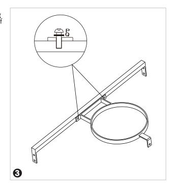
Attach Tank Support Bar ① to Door Frame Leg ② and Support Leg 1 ② by aligning holes at each end of Tank Support Bar with holes at the bottom of Door Frame Leg and Support Leg 1. Place a Washer ② on each of four Bolts ② and insert into holes. Tighten with Hex Key ③.
