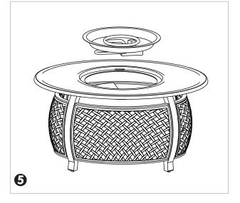
6 Pour the Fire Class • around the Burner. Be careful not to obstruct pilot light housing. Put the Removable Burner Cover • on the Burner.
