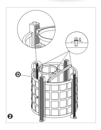
Place Table Top so underside faces up. Screw 4 Studs into the holes on the Table Top with Screwdriver . Then carefully turn the assembled fire pit base upside-down and align the holes in the top of the Legs with the Studs in the Table Top.
