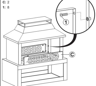
Align two Decorative Panels (C) with the side panels and secure using four M6x12mm Bolts (1), as shown.
