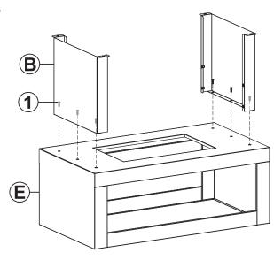
Align two Side Panels (B) with Base (E) and secure using six M6x12mm Bolts (1), as shown.
