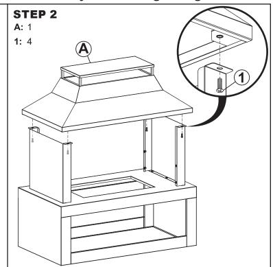
Align Lid (A) with the side panels and secure using four M6x12mm Bolts (1), as shown.
