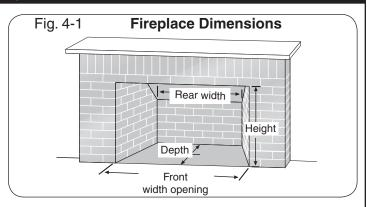
Note: It is recommended that complete firebox dimensions (front width, back wall, and height) be obtained to ensure proper sizing.
