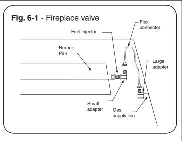
appropriate soapy water solution. If bubbles appear, a leak is present. Turn off the gas and tighten at all connections. Repeat until no leaks are present. If a leak persists, turn off the gas supply and contact the local gas company or dealer. NEVER USE A FLAME TO CHECK FOR LEAKS.
