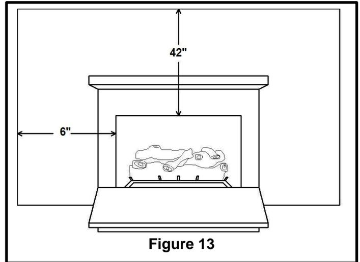
These dimensions are **MINIMUM CLEARANCES** to maintain when you install this burner system. The fireplace opening **MUST BE AT LEAST 6"** from any combustibile sidewall. The ceiling **MUST BE AT LEAST 42"** from the top of the fireplace opening.
