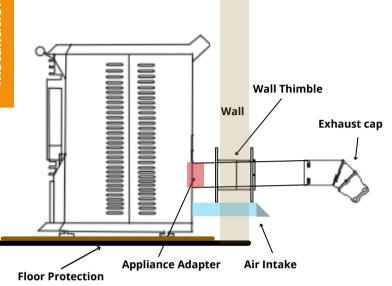
**Notice:** Excessive embers/sparks can exit exhaust cap if less than 4 ft of venting is used with no vertical rise.
