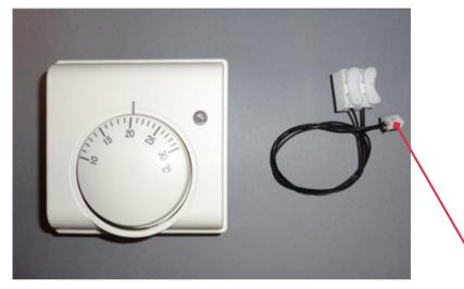
**Connecting a Thermostat:** Connect the "Call for Heat" extension wires from the thermostat to the bottom circuit board.
