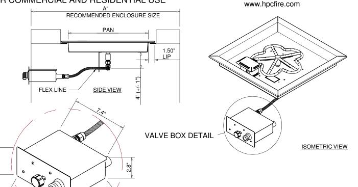
SPARK IGNITION BY AA BATTERY MATERIAL: 304 STAINLESS STEEL
