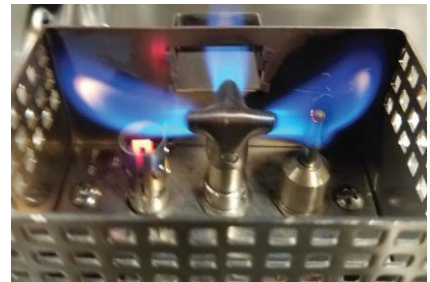
Figure 10.2 – Pilot flame coverage of thermocouple.
