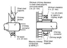
D Solid-insulated, listed factory-built chimney length with an inside diameter 2 in. (51 mm) larger than the chimney connector and having 1 in. (25 mm) or more of insulation, serving as a passthrough for a single wall sheet steel chimney connector of minimum 24 gauge [0.024 in. (0.61 mm)] thickness, with a minimum 2-in. (51-mm) air space between the outer wall of chimney section and combustibles.
